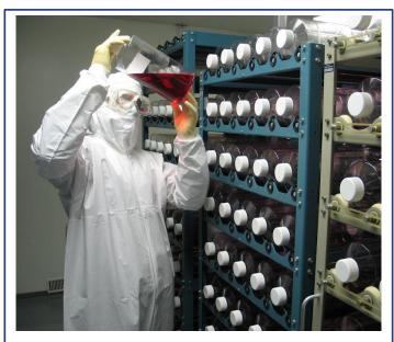
Microbix' expertise in large-scale roller bottle cultures remains a mainstay of its production process even as bioreactor culture ramps up for key products.
