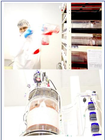
Microbix's expertise in large-scale roller bottle culturing (upper frame) remains a core skill, while our bioreactor culturing (lower frame) further improves process control and yields.
